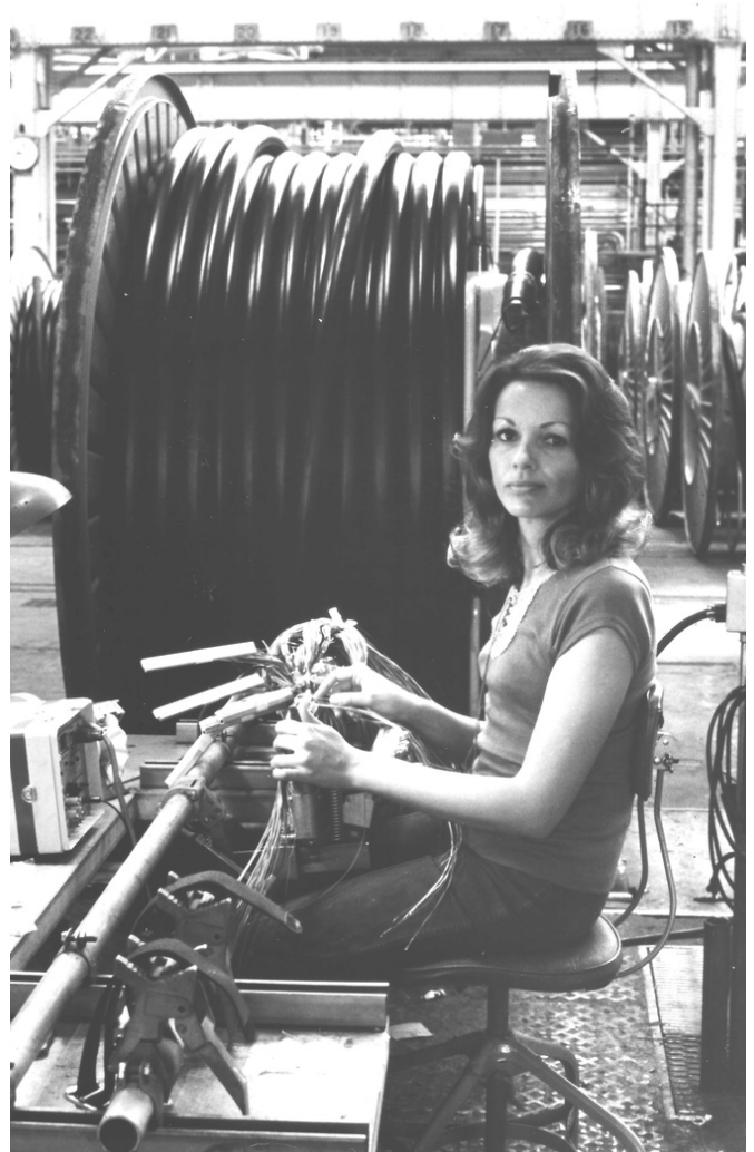
Western Electric Woman Splicing Cable, courtesy of Baltimore Museum of Industry Archives.
